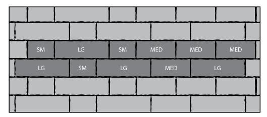
Install Eurostone pavers randomly or simplify installation by repeating the 11-paver pattern shown above (3:4:4 ratio) to create a random appearance.
